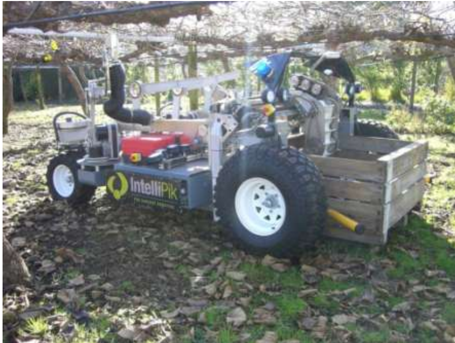
Figure 1 Autonomous chassis configured for picking with four robot arms but only one picking hand
